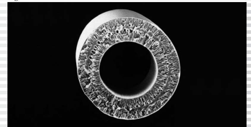
Hollow fiber ultrafiltration medium shown at 300X magnification
